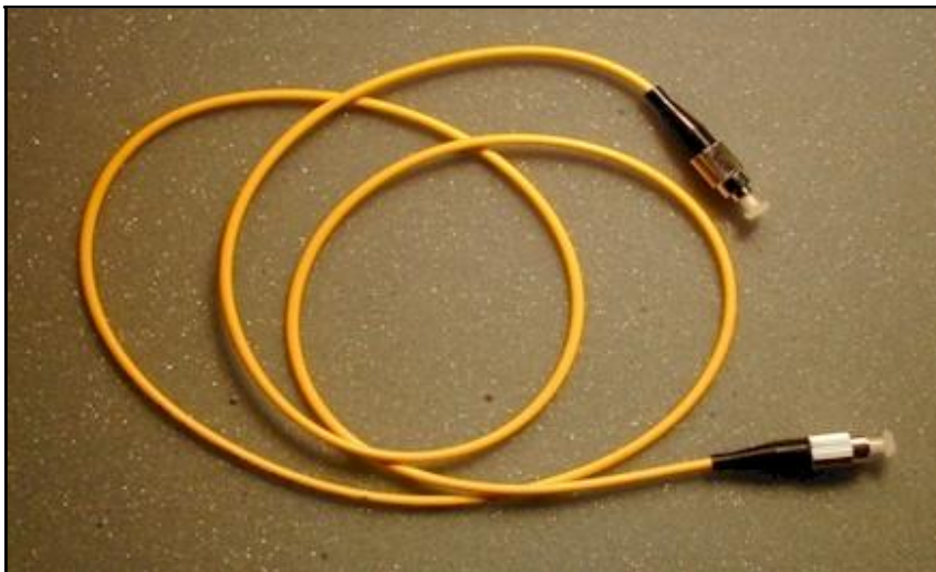
Figure 1. Fiber optical reflection reference patchcord
