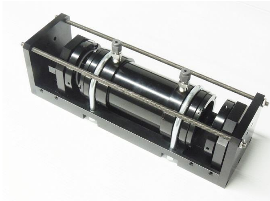
OESEN-LPC-100 Gas Cell with built-in isolated chamber
