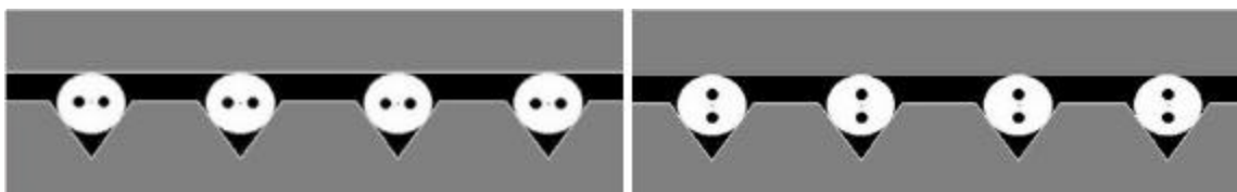
PM fiber array aligned with fast axis and slow axis
