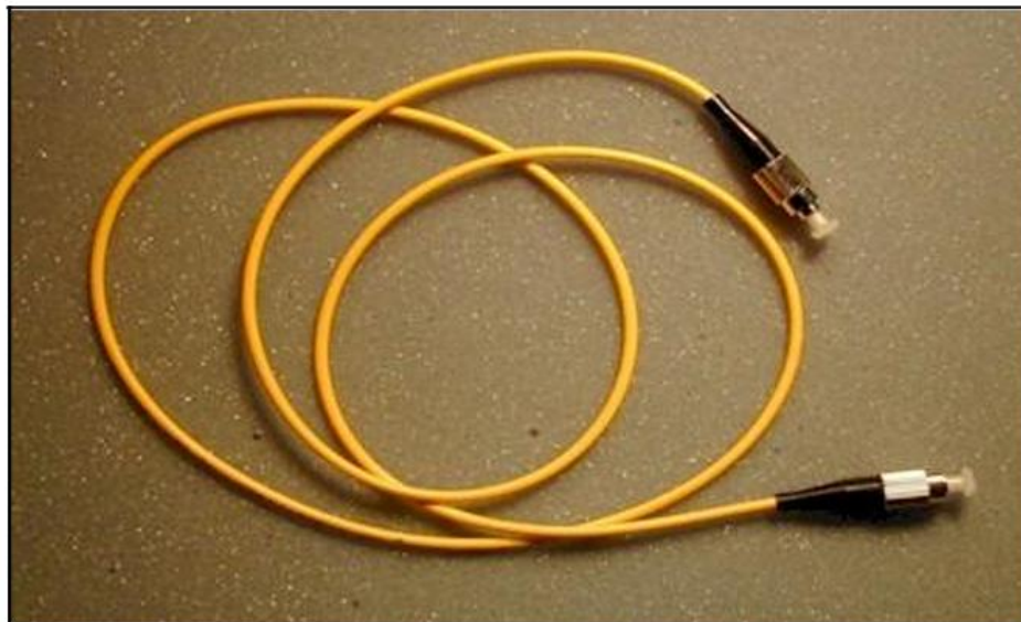
Fig.1 Fiber optical reflection reference patchcord
