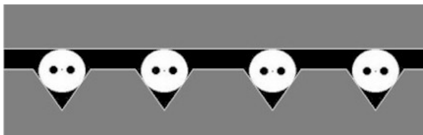
Fig 2. A 4 channel PM fiber array with fast axis alignment
