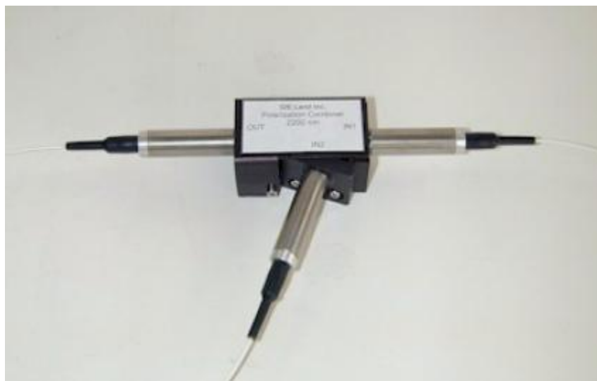
Fig1. Free space optics based fiber polarization combiner
