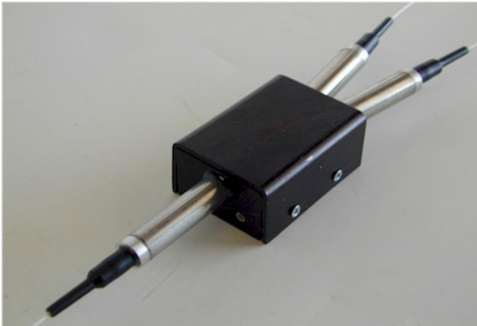
Fig1. Optical fiber Polarization Splitter
